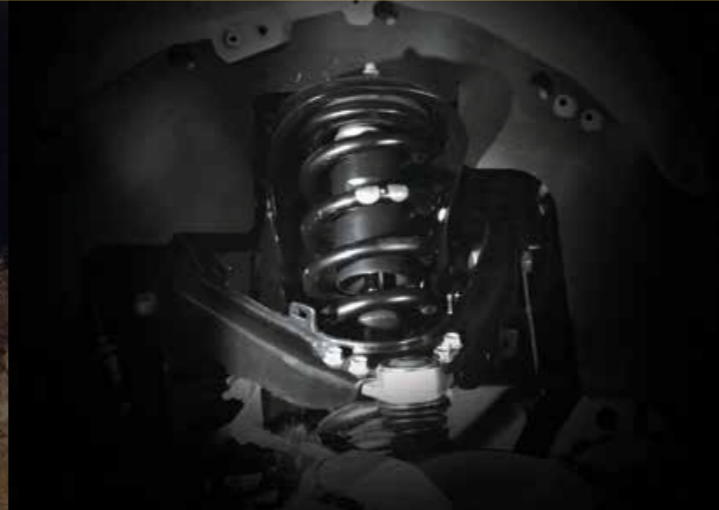
Independent high ride front coil spring suspension with gas shock absorbers, stabiliser bar, upper and lower wishbones
