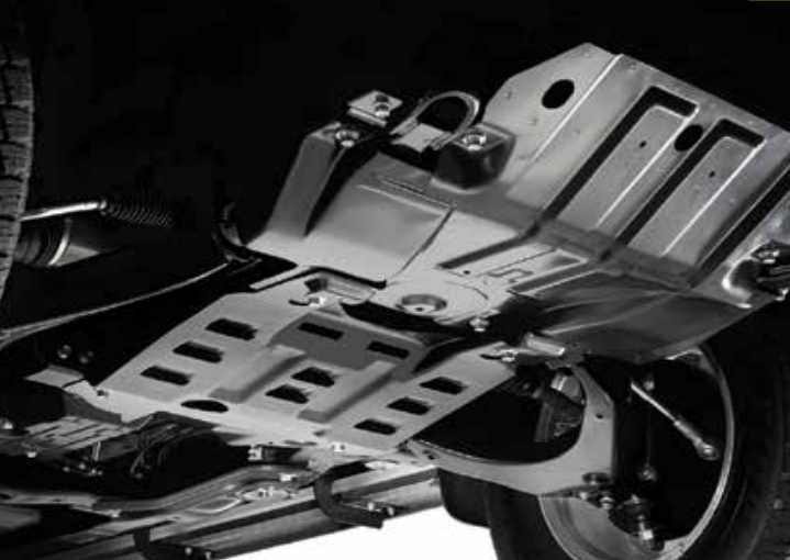
Underbody protection, front steel plate skid/shield
