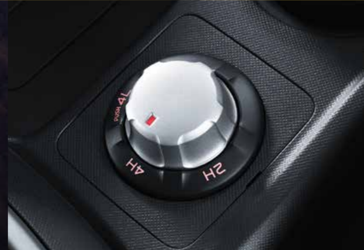
"Terrain Command" 4WD system allows for simple shift from 2WD high, 4WD high and 4WD low
