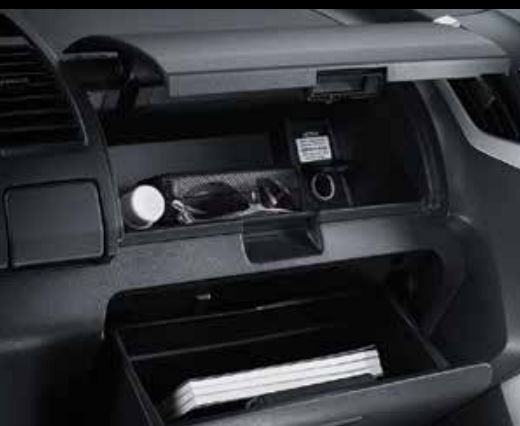
Glove compartment (lower) and article storage compartment (upper) with easy access power outlet
