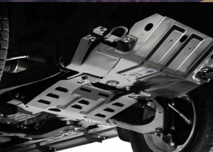
Underbody protection, front steel plate skid/shield
