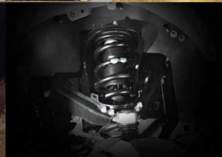
Independent high ride front coil spring suspension with gas shock absorbers, stabiliser bar, upper and lower wishbones
